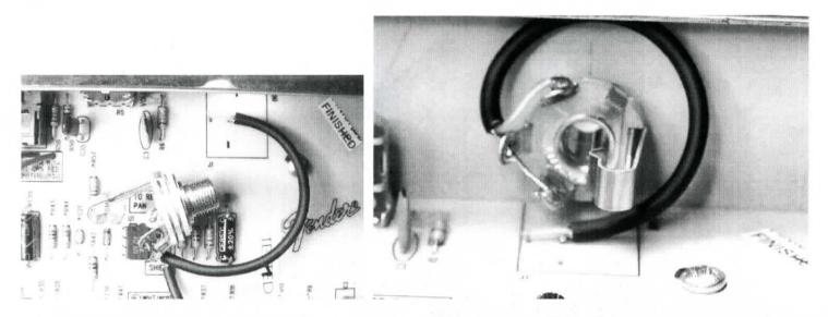
On the green board, clip jumper W25 and solder the center lead to R1 and the shield to R2, as shown. The green board has no shielding on the board, so running directly to the input resistor makes the amp quieter and prevents internal feedback from the treble control.
