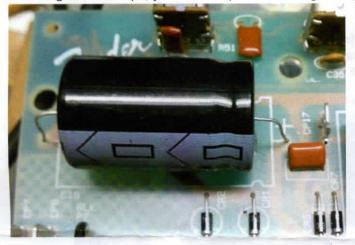
cleanly. Note that the rev B green board uses a longer, 500V cap. All other BJrs use a 450V cap, which has plenty of safety margin; the plate voltage is only around 330V.
