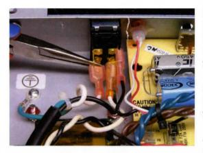
2. Remove the push-on disconnects from the power switch. Long-nose pliers or a slim screwdriver may help get things moving. Then remove the stock power switch with a 9/16" socket wrench or nut driver. Don't use pliers—you'll scratch the faceplate for sure.
