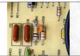
Clip the leads of R51 and R52 flush with the board. The stubs are easier to desolder and thereby prevent damage to the traces. A vacuum plunger desolderer (solder sucker) is highly recommended.
