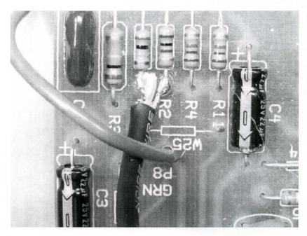
shield lead goes in there and the center lead goes into the vacant W25 hole that leads to the input resistor.
