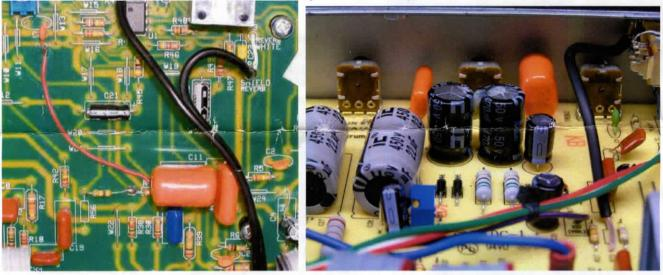
On the green board, you can also see the reverb mod. I like to put a small dab of hot melt or silicone glue between the tone caps to ensure that they won't vibrate against one another.
