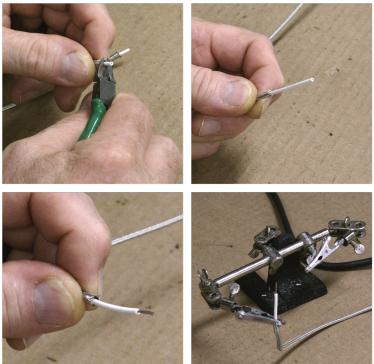
Slide the RCA plug over the stripped cable and solder the wire to the tip. Flip the cable upside down, push down the braided shield so it touches the sleeve of the RCA plug. Quickly solder the shield to the sleeve to avoid shorts from overheating the wire's insulation.
